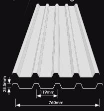
Cover width: 760mm Total width: 810mm Coil width: 925mm All dimensions given are nominal Minimum Pitch 7.5° (approx. 1:7.5)
